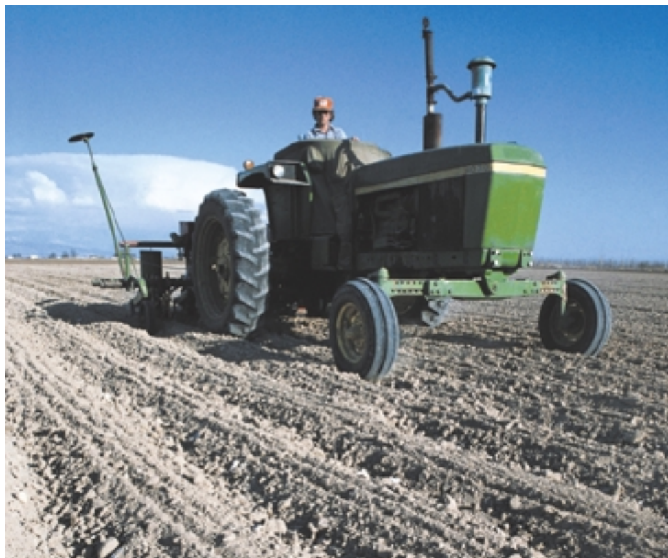
Figure 2.71 Zero-tillage cultivators cut weeds near the soil surface, disturbing it as little as possible.
