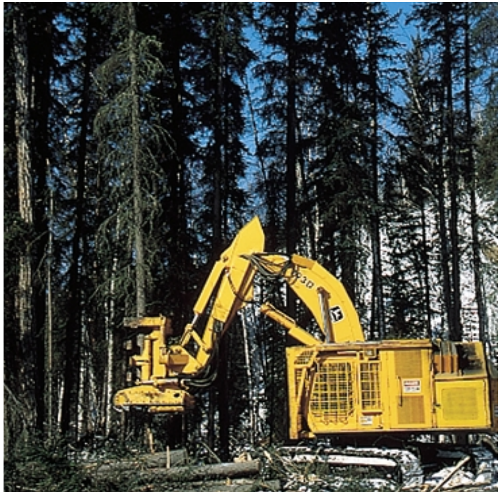
Figure 2.49 Feller-bunchers like this one are replacing the axe and chainsaw methods of the past. This machine quickly cuts down the trees. A separate machine called a de-limber and processor removes the branches and cuts them to log length. A powerful rotary (or circular) saw uses hydraulic technology to cut the trunk.
