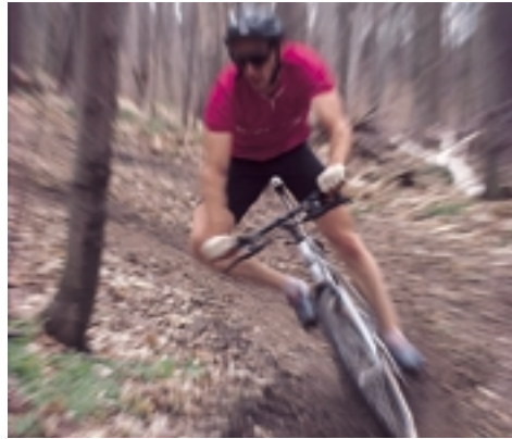
Figure 4.69A Rapidly spinning wheels stabilize a bicycle.
