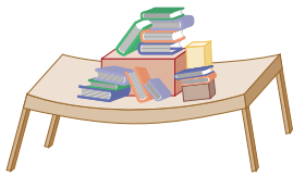
Figure 4.51 When a horizontal structure carries a heavy load, it may begin to sag in the middle.
