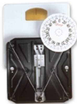
Figure 4.33 A standard bathroom scale is a type of spring scale. Springs within the scale are stretched when a person stands on the scale. The springs are connected to parts that move a numbered scale below a fixed needle.
