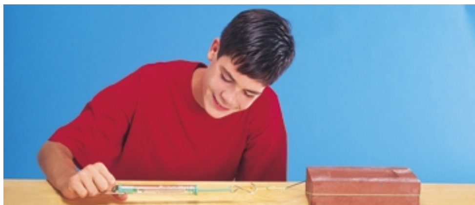
Figure 4.32 A force can be measured by seeing how far it stretches the spring in a force meter.
