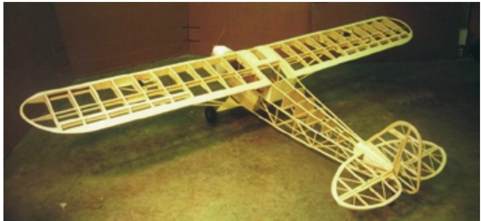
Figure 4.11 A flimsy framework of balsa wood, covered with painted tissue paper or plastic film, makes a model aircraft strong enough to take off, do complicated stunts, and land safely.
