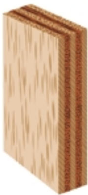
Figure 4.19 How do plywood laminations add strength to the wood?
