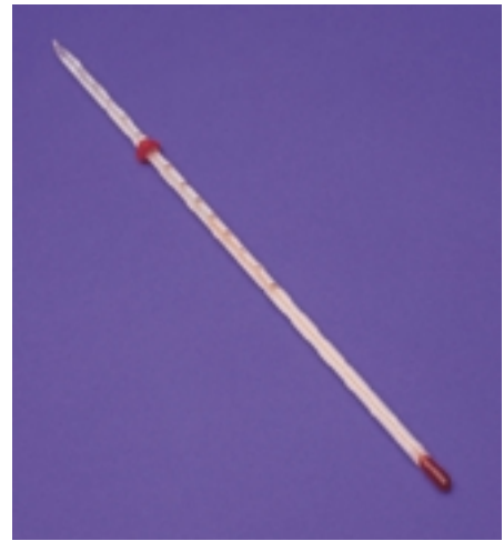
Figure 3.4C A modern laboratory thermometer has a smaller bulb and a much narrower opening in the glass stem.
